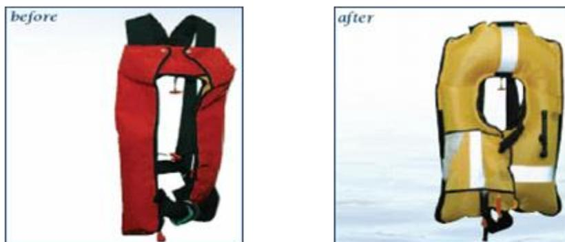
**Pouch style** – A pouch style PFD can be inflated manually (by pulling a toggle to activate CO<sub>2</sub> inflation) or inflated orally (by blowing into a tube). The pouch style PFD is considered a 2-stage donning device because once the inflation mechanism is triggered, the inflated chamber comes out of the pouch and then the wearer must pull the inflated chamber over his or her head to correctly wear the inflated PFD.
