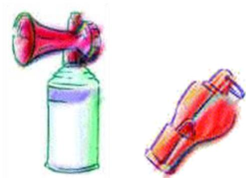
**Sound Signalling Devices** – All vessels under 12 m (39.4 ft.) in length and not equipped with a sound signalling appliance must carry some type of sound signalling device (such as a pealess whistle or a compressed gas horn).
