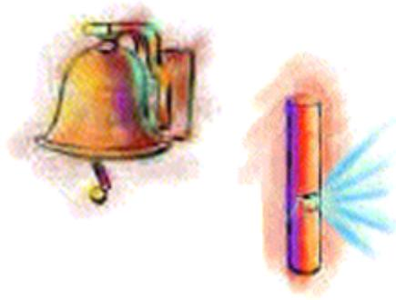
**Sound Signalling Appliances** – Vessels that are 12 metres or more in length must carry a sound signalling appliance (such as a bell and whistle). Vessels that are 20 (65.6 ft.) metres or more in length must be equipped with two sound signalling devices (one of which must be a bell). Sound signalling devices must meet technical criteria for frequency and audible range as described in the *Collision Regulations*:
