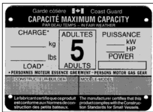
In Canada, any pleasure craft that is propelled (or designed to be propelled) by a motor is required by Transport Canada to carry a label, tag, or plate called a “**Compliance Notice**”. The Compliance Notice must be permanently affixed to the hull of the vessel, usually at the back of the vessel, in a location where it can be read from inside the vessel.
