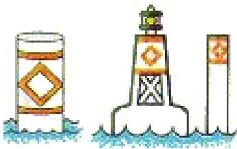
A **hazard buoy** marks local water hazards such as rocks and shoals. This type of buoy is white in colour and is marked with a hollow orange diamond symbol with two horizontal orange bands, one above the diamond and one below. Information concerning the hazard is indicated by a black symbol displayed inside the orange diamond. If it carries a light, the light is yellow in colour and operates on a flash cycle, (F1) 4s, (i.e. flashing once every 4 seconds).
