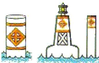
A **keep-out buoy** is used to mark an area in which boats are prohibited. It is white in colour and is marked with a hollow orange diamond symbol the interior points of which are joined by an orange cross. It also has two orange, horizontal bands, one above and one below the diamond-shaped symbol. If it carries a light, the light is yellow in colour and operates on a flash cycle, (F1) 4s, (i.e. flashing once every 4 seconds).
