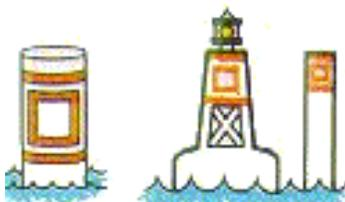
An **information buoy** displays by means of words or symbols information about a locality, marina, or campsite. This type of buoy is white in colour and displays information within a hollow orange square with two horizontal orange bands, one above the square and one below. Information about a locality is displayed with black symbols inside the square. If this buoy carries a light, the light is yellow in colour and operates on a flash cycle, (F1) 4s, (one flash, repeated every 4 seconds).
