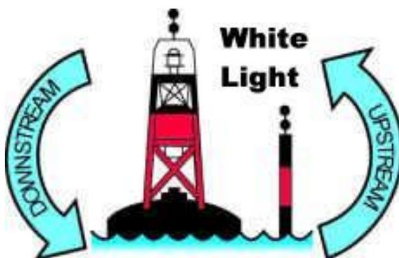
**navigable water all around it. To be safe, stay well away from this type of buoy.** Consult your marine chart for details on the nature of the danger (dimensions, depth, etc). This buoy is painted black with a horizontal red – coloured band midway up. If equipped with a light, it will be white in colour and will operate on a flash cycle (giving two flashes every 4 seconds).
